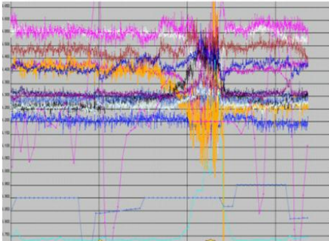
Figure 3. Elvis Web 2.0 interface: current of individual anodes.
