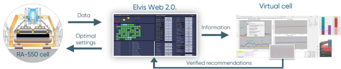
Figure 1. Interaction of the virtual cell with the physical RA-550 cell.
